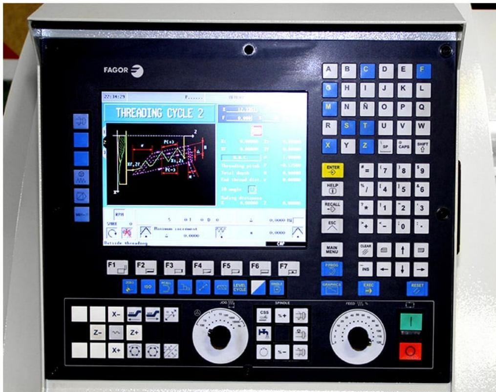
The control language is conversational or G-code, with on-screen menus and prompts to make programming virtually foolproof. The Fagor control offers a teach in mode. Moving the machine to produce the part manually and then with a few simple key strokes the control stores these movements as a machining sequence and creates the part program for use. At a later time, retrieve the program, enter the number of parts to be produced, and your Fagor control does the rest.
